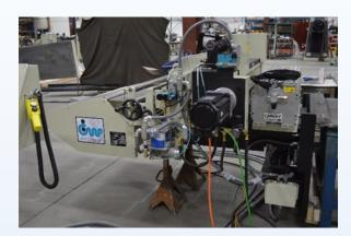
The line includes a 20,000 lb. capacity uncoiler with secondary coil clamping arm for safe thread-up of high yield materials, automatic brake tension control, and coil loading car.
