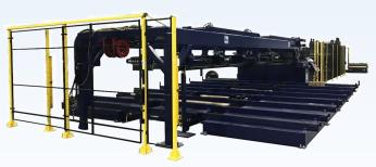
with Pallet Staging. What is unique to this line is the ability to stack up to 338" blanks, and longer blanks will process with end discharge as needed for future manufacturing needs of the customer. Added to the Morgan Olson facility in late February was our 20,000 lb. Upender to allow coils that are delivered eye-to-the-sky to be oriented for loading onto the Cut-to-Length System.
