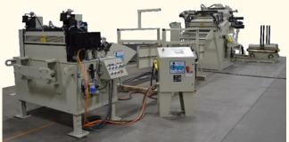
loading car, allowing loading and off loading of partial coils. The Reel and Straightener are complimented by the Hold Down Peeler System and Secondary Hold Down Arm to safely handle the thicker material during thread up. Smooth Chrome Straightening Rolls and Powered High lift head allow ease of roll cleaning. Our SMX36H6 ServoMax Feed features Handwheel Edge Guides, Anti-backup Rolls, Auto Lubrication and Powered Passline Height Adjustment.
