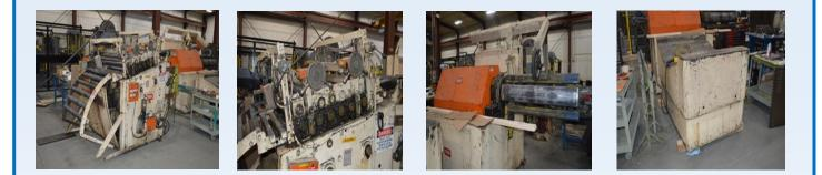
The unit was thoroughly cleaned and the straightener head was disassembled. All bearings, rolls, sprockets, gears, chains, and guards were inspected and replaced as needed. The new motors and controls were installed, programmed, and tested. The unit was painted using our standard colors to best match the original colors of the equipment (Formtek-Beige and safety orange).
