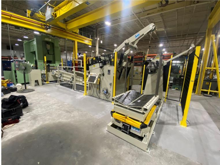
The system includes a 15,000 lb. stock reel equipped with a 2-pressure brake system for regulated pressure in run mode and full-pressure for e-stops, automatic brake tension control to adjust brake pressure automatically as the coil depletes, coil O.D. capacity up to 72", and bolt-on coil arm spacers to provide an auxiliary expansion range beyond the standard 17.5" to 22.5".
