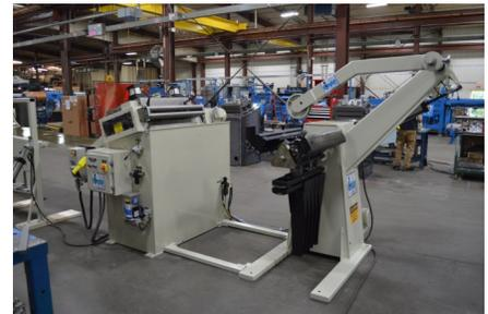
The ServoMax feed is equipped with 460/3/60 voltage, automatic central lubrication, and an adjustable height cabinet. The unit includes our standard B&R control platform.
